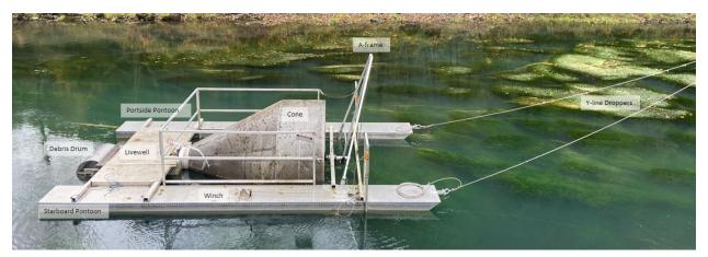
Figure F-1. Labelled image of a rotary screw trap showing parts and terminology.
